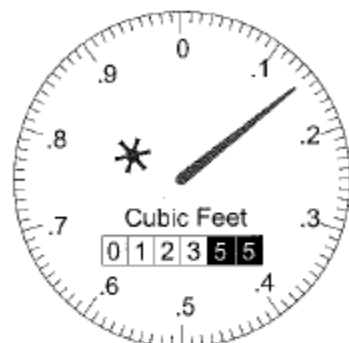
Meter indicating 123 Ccf. Leak indicator is shown in blue.
